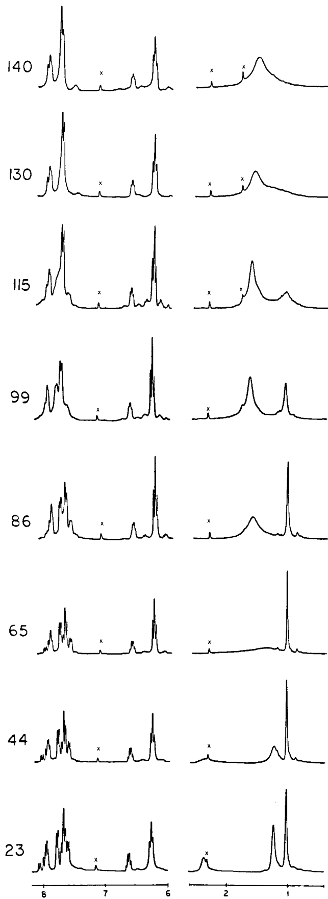
Figure 4. 1 H NMR spectrum in C 2 D 2 Cl 4 (80 MHz) of [\text{B}(\text{pz})_4]\text{-TaMe}_3\text{Cl} at various temperatures (°C). The × peaks are due to residual toluene and sample decomposition.
